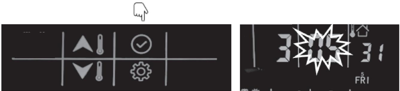
6. Next, press the “up” or “down” button to set the correct time in minutes;
