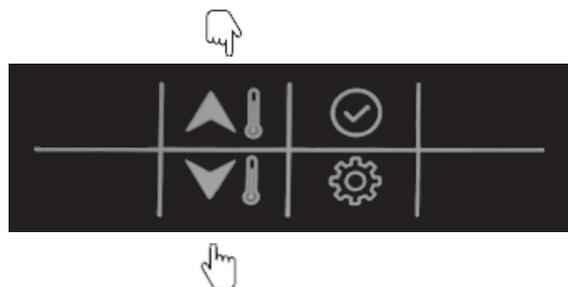
5. After setting the hour, press the “confirm” button to enter the “minutes” setting; the minutes will flash at this moment.
