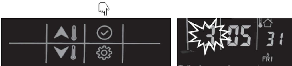
4. Next, press the “up” or “down” button to set the correct time in hours;
