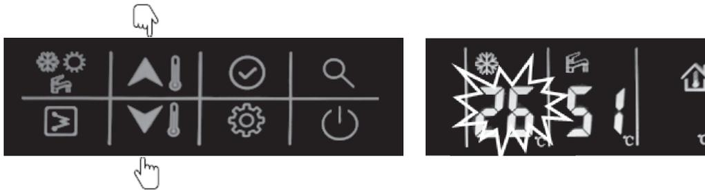
ii. Next, press the confirm button or wait for 5s without pressing any button to change the DHW temperature setting. Next, press the “up” or “down” button to change the DHW.
