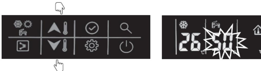
ii. Press the confirm button or wait for 5s without pressing any button to enter the setting value of LWT. Next, press the “up” or “down” button to change the air setpoint.
