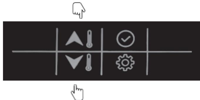
7. Press the “confirm” button to confirm and exit clock settings. You can also press the “settings” button to go to the next parameter. (Refer to the user parameter configuration for the full details on parameters setting)
