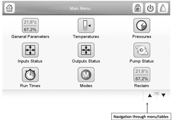
Specific unit parameters table/menu can be accessed by pressing the icon corresponding to the desired category. In order to go back to the Synoptic screen, press
