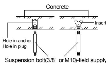
2.2.3 Install the suspension bolts (use W3/8 or M10 suspension bolts, 4 pieces) depending on the ceiling type.
