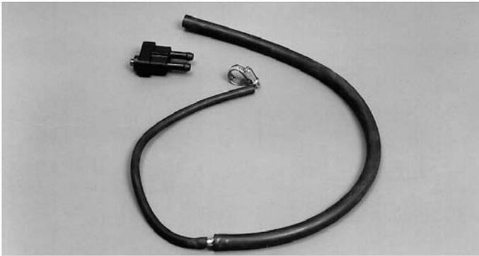
1. Remove the rubber plug from the plastic base of the thermostat to enable the 3/16 in diameter tube from the warm-up switch to be connected.
