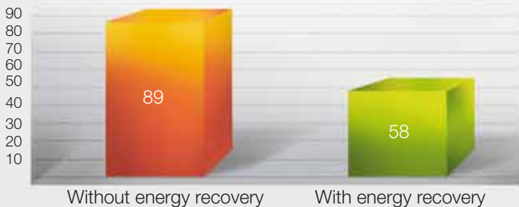
Simulation performed for an office building (1380 m 2 ) with Carrier's HAP software kWh/m 2 /year
